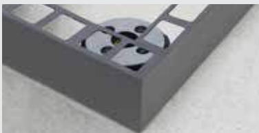
F2. Slide the BSRE joint profile along the BSR profile. Place the composed piece on the pedestal.
