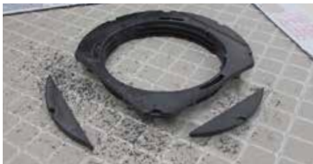
1. Turn the base upside down and remove two sides along the marked lines.
