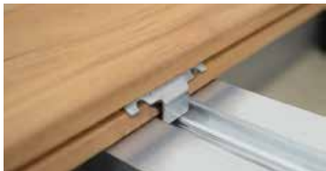
20. Position a SUPCLIP clip to block the boards.
