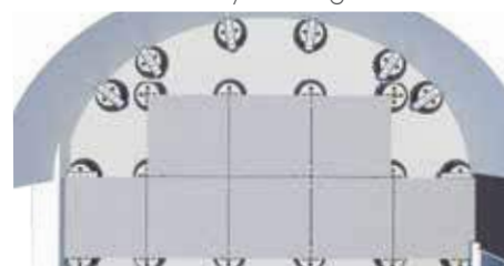
14. Place the tiles following the layout diagram.
