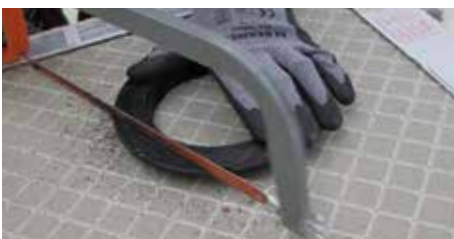
3. Turn the base upside down and remove one of the sides along the marked line.
