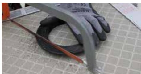
7. Turn the base upside down and remove one of the sides along the marked line.
